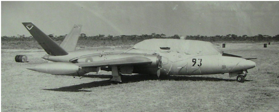
Fig 4. The Fouga CM 170 "Magister" #93 at Kolwezi Air Base, with nose-mounted guns and wing-tip tanks.
